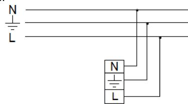
2. Mains connection scheme for luminaire with 1-10V or DALI regulated control gear.
